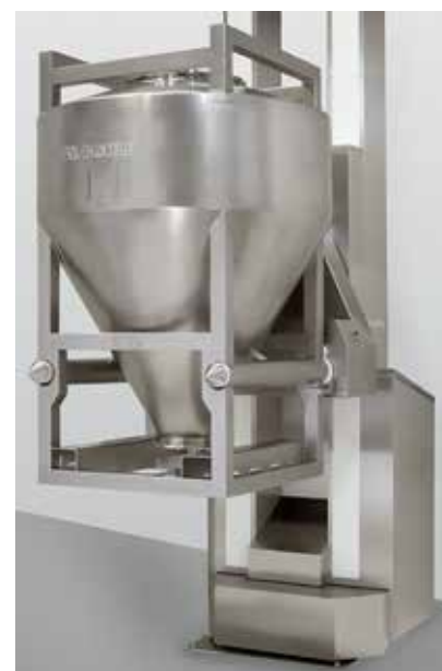
Figure 2: Exemplary container blender (source: L.B. Bohle).
